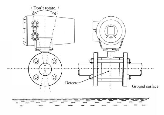
Figure 4.6 Installation position of the detector
